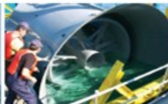
Submerged Ducted Rim Sea testing at Race Rocks, BC, Canada (Clean Current Power Systems Incorporated, Canada)
