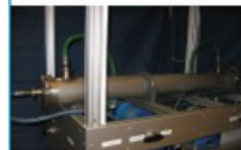
Experimental set-up for membrane development for harnessing salinity gradient energy Osmotic Power (Statkraft SF, Norway)
