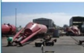
Pelamis Floating, articulated device Assembling of the first offshore wave farm off Northern Portugal (Ocean Power Delivery, UK)
