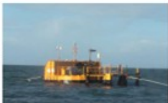
OE Buoy Floating OWC system Sea testing in Galway Bay Test Site, Ireland (Ocean Energy Ltd, Ireland)
