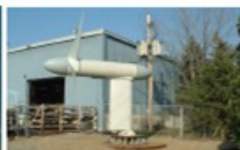
Kinetic Hydro Power Systems (KHPS) Turbine tested in East River, USA (Meridian Power, USA)
