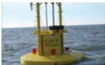
PowerBuoy Free-floating point absorber Sea testing in Hawaii (Ocean Power Technologies, USA)
