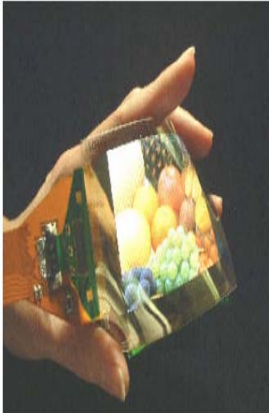
Pioneer in SID'03. 3", 8 bits grey scale 160xRGBx120 SiON passivation layers
