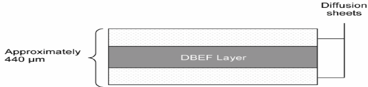
Structure of a brightness-enhancing film Source: 3M's DBEF-D document
